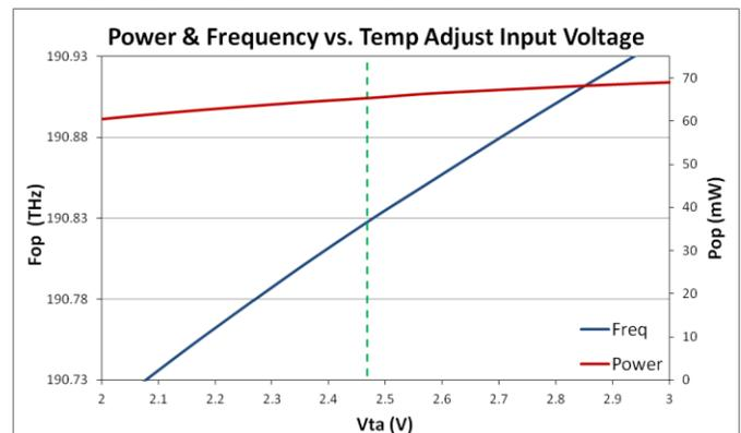
**Figure 1: Variation in output frequency and power as a function of temperature adjust input voltage for a 63mW 1571nm EM650. Typical mode hop free tuning range is  $\pm 50$  GHz from the default operating point. The dashed green line represents the  $V_{ta}$  open circuit voltage.**
