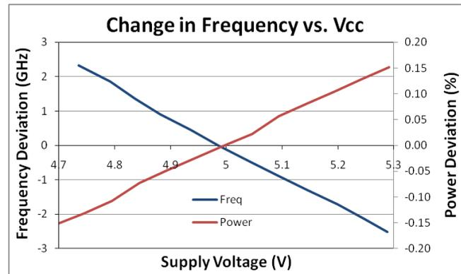
**Figure 3: Frequency and power deviation as a function of supply voltage.**
