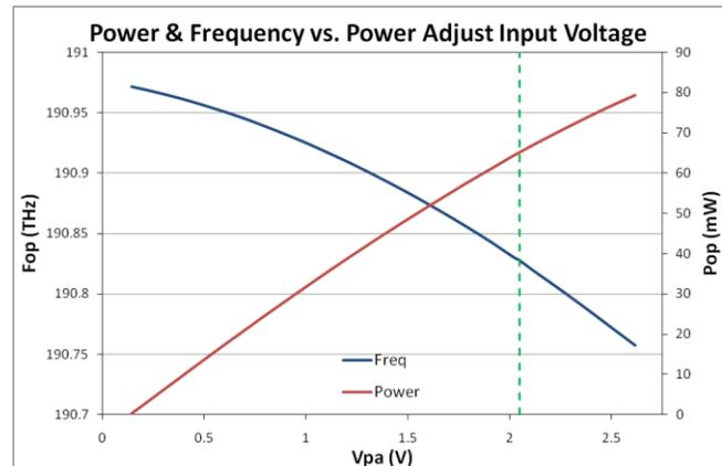
**Figure 2: Variation in output power and output frequency for a 63mW rated 1571nm EM650 using the power adjust input. The dashed green line represents the Vpa open circuit voltage. Note some devices may exhibit a mode hop (frequency shift) as power increases. Typical mode hop free tuning range is ±50GHz from default operating point**
